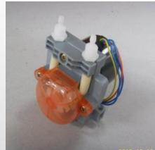
DETERGENT Pump(Motor) Dispense the chemical agent to wash tank as programmed time (6~20sec.) Made of chemical resistance material. \* When M/C work by door closed, dispenser also work as program at washing procedure. SPECIFICATIONS a. Rated revolutions : 49 rpm b. Electric power : 220V 1Ph c. Power consumption : 7 W d. Dispense time : 6 ~ 20sec.(8stage), 6~20cc
